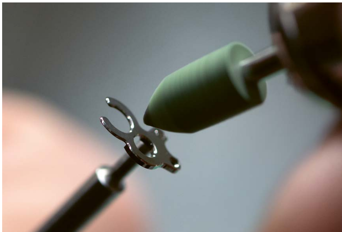
Top left: Satin finishing of the flank of a minute train bridge using a micromotor with a diamond point. Above: Buffing of the angles of a minute train bridge using a micromotor with a finishing rubber.
