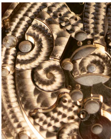
Hand circular-graining of a plate.
