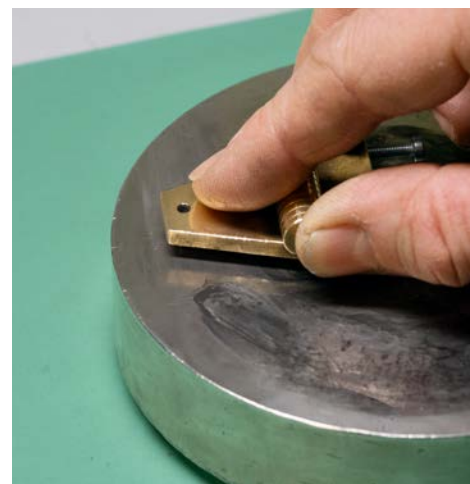
Bridge of the split-seconds wheel ready to be polished, placed in its support.
