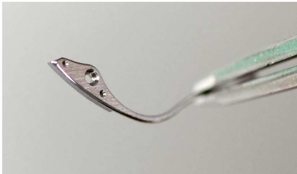
Operating lever spring finalised after straight-graining.
