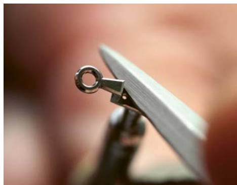
Chamfering a flying "égalité" bridge with a file.
